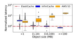
**Figure 16:** Normalized latencies grouped by object sizes. Each is normalized to that of ElastiCache.
