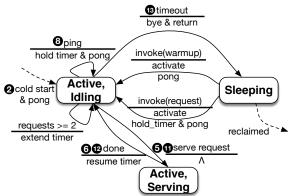
Figure 7: State transitions of a Lambda function runtime.
