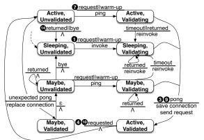
Figure 6: Lambda connection validation process in a proxy.
