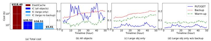
Figure 13: Total \$ cost (a) for ElastiCache and INFINICACHE (IC), and INFINICACHE's hourly cost breakdown under various settings (b)-(e).
