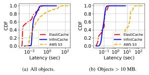
Figure 15: INFINICACHE latencies vs. AWS S3 and ElastiCache.
