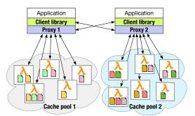
**Figure 2:** INFINICACHE architecture overview. Icon denotes EC-encoded object chunks. Chunks with same color belong to the same object.
