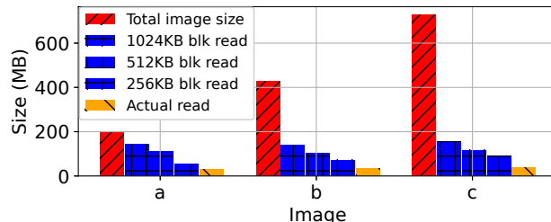
Figure 20: Amounts of data fetched (on-demand) as a function of block sizes. Left-most bar in each bar cluster represents the size of the original container image; right-most bar in each bar cluster represents the actual amount of data read from the data blocks fetched via network.
